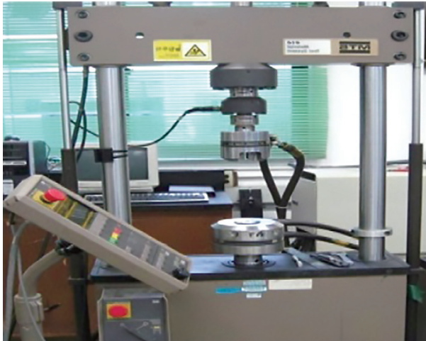
Fig 4: Dynamic loading fatigue tester
