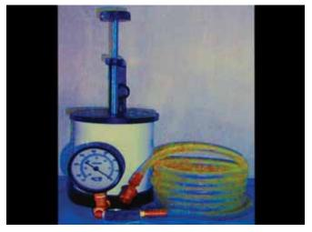
Fig. 7: Custom-made vacuum chamber used for the study
