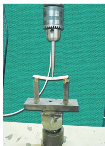
Fig. 2: Flexural strength testing in universal testing machine
