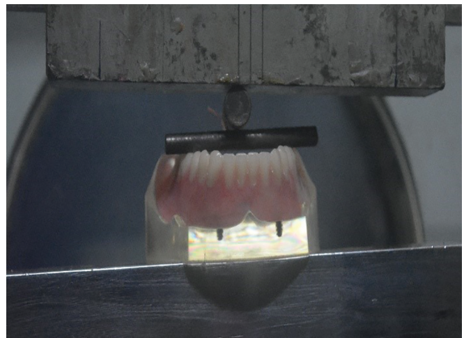
Fig. 1: A photoelastic model with a mandibular overdenture positioned individually in a circular polariscope adapted to a universal testing machine with an axial load of 15 pounds applied bilaterally to the central fossa region of the first molar
