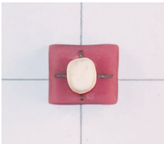
Fig. 2: Custom-fit bases marked to ensure reproducibility of the tooth and die position
