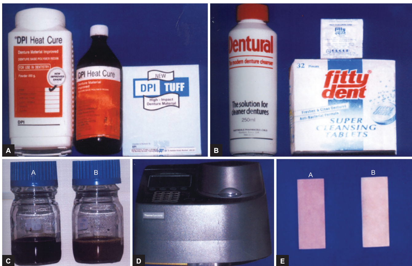
Figs 1A to E: Materials used in the study. (A) Denture base resins; (B) cleansers; (C) staining solutions (a, tea solution and b, paan solution); (D) spectrophotometer; and (E) specimens (a, conventional and b, high impact)
