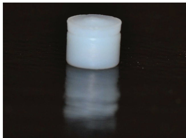
Fig. 2: Teflon sleeve-encased dental magnet
