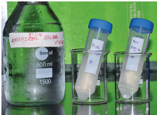
Fig. 3: Control and test magnets dipped in artificial saliva
