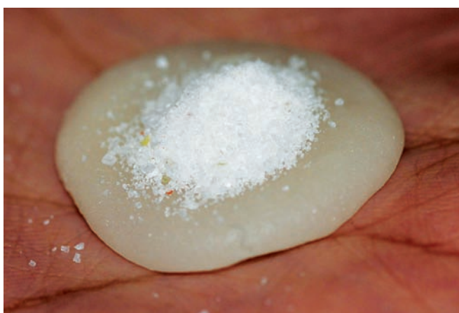
Fig. 6: Packing of the heat cure PMMA with salt crystals between two layers
