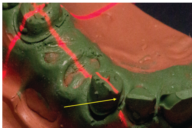
Fig. 6: Noncontinuous laser line on one of the axial walls (yellow arrow) indicating the presence of an undercut
