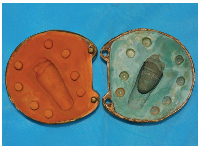
Fig. 8: Dewaxing of the wax pattern
