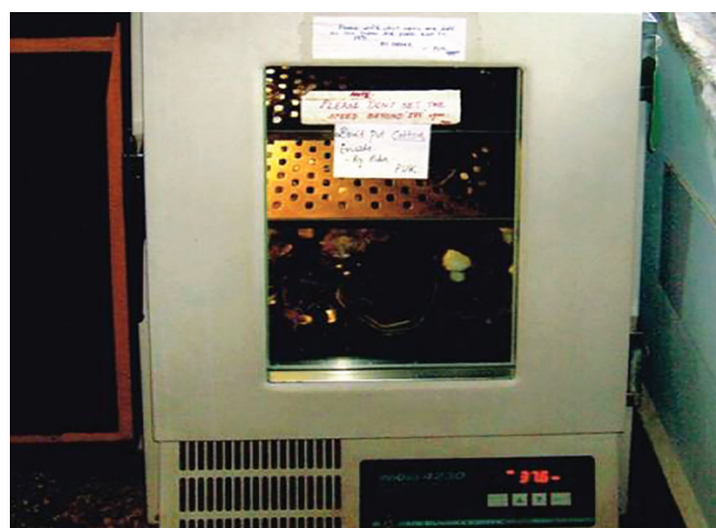
Fig. 3: Environmental chamber with temperature control used for weathering study group specimens of silicone and heat-cure clear acrylic resin
