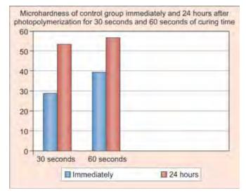
**Graph 5:** Microhardness values (VHN) of group A, for subgroup  $t_{30}$  and  $t_{60}$ , immediately and 24 hours after photopolymerization
