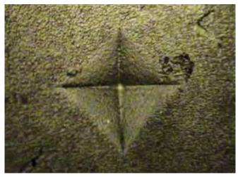
Fig. 6: Microscopic image of indentation at 40× magnification
