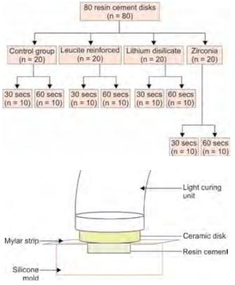
Fig. 3: Schematic diagram of the experimental set-up to irradiate specimens through machinable ceramic
