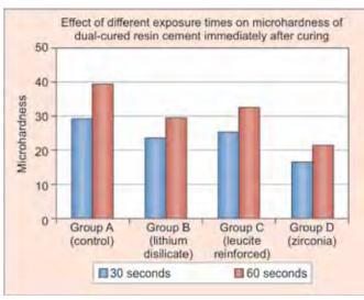
**Graph 3:** Microhardness values (VHN) of groups A, B, C and D for subgroup  $t_{30}$  and  $t_{60}$ , immediately after photopolymerization
