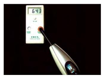
Fig. 2: Radiometer showing the light intensity
