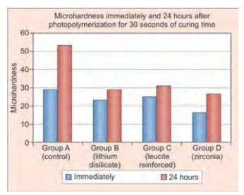
**Graph 1:** Microhardness values (VHN) of groups A, B, C and D for subgroup t<sub>30</sub>, immediately and 24 hours after photopolymerization
