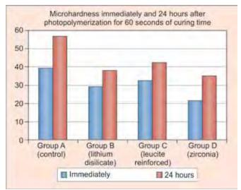
**Graph 2:** Microhardness values (VHN) of groups A, B, C and D for subgroup t<sub>60</sub>, immediately and 24 hours after photopolymerization
