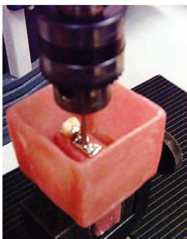
Fig. 9: Cobalt-chromium clasp attached to the universal testing machine
