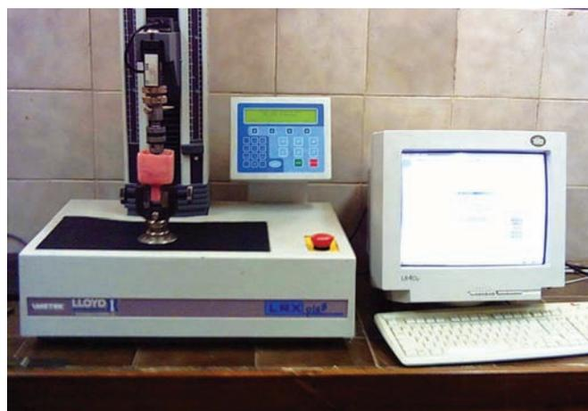
Fig. 10: Universal testing machine
