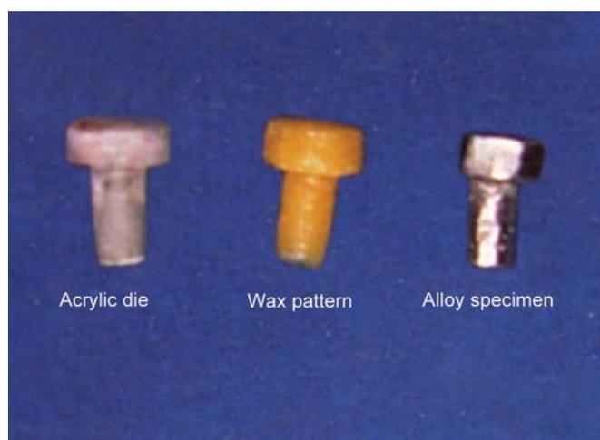
Fig. 1: Die, pattern and casted specimen
