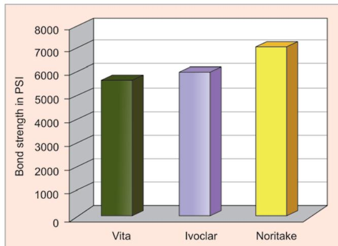
**Graph 2:** Comparison of bond strength between recast alloy and various ceramics
