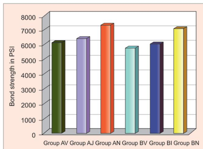
**Graph 3:** Comparison of bond strength between alloys and various ceramics
