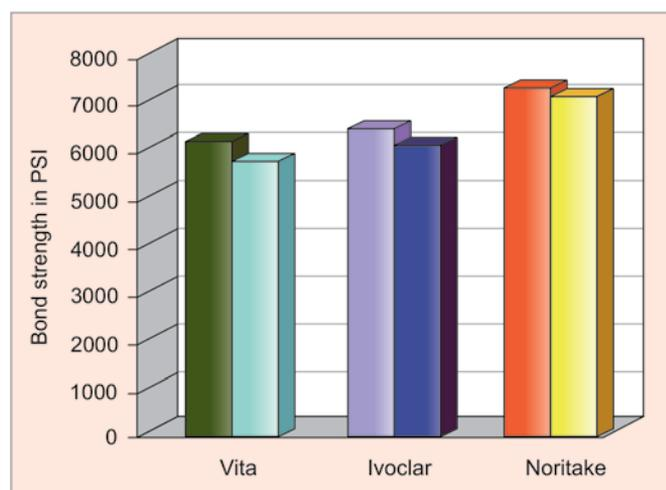
**Graph 4:** Comparison of bond strength between 100% and recast alloys using various ceramics
