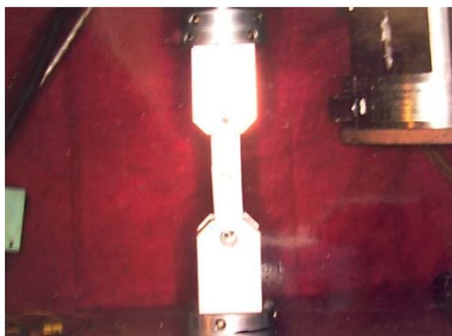
Fig. 2: Specimens with attachments mounted on MTS
