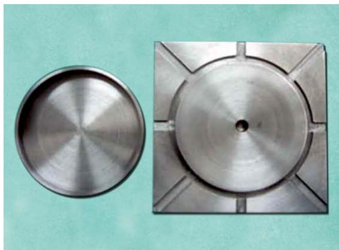
Fig. 1: The master die and the milled metal spacer of 2 mm thickness
