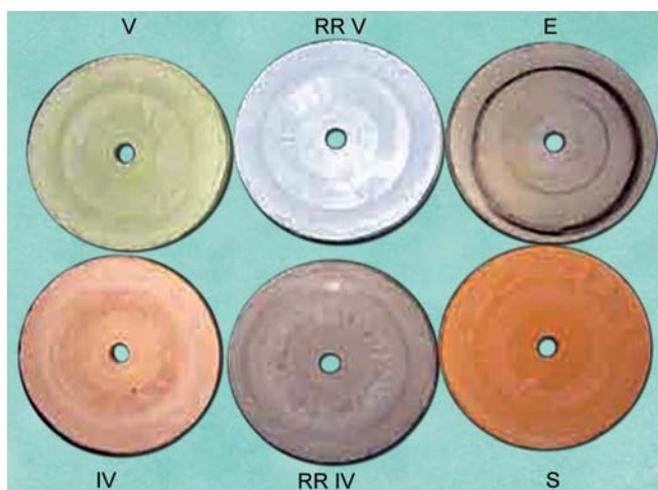
Fig. 3: Samples for the abrasion resistance test. Materials are identified by their color and code
