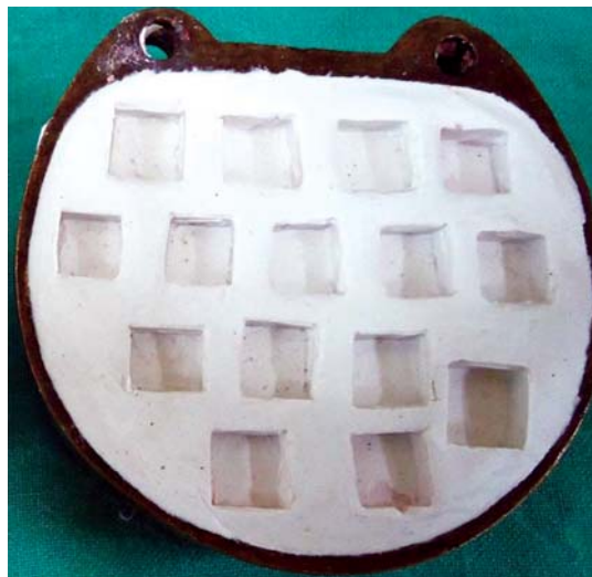
Fig. 1: Stone mold for preparation of specimens in hanau flask
