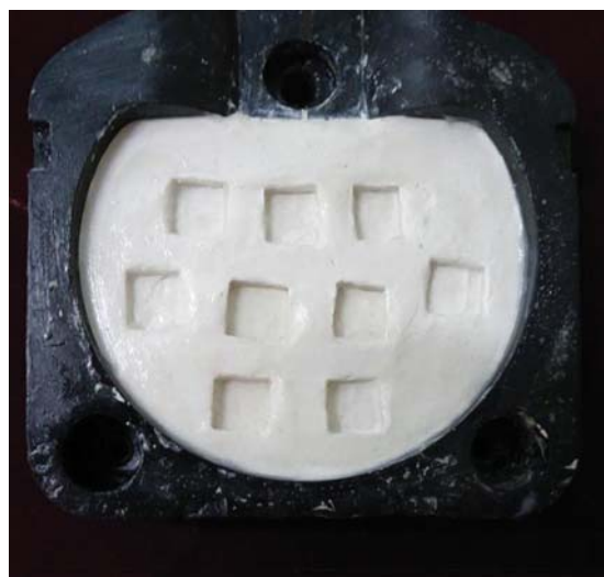
Fig. 2: Stone mold for preparation of specimens in FRP flask
