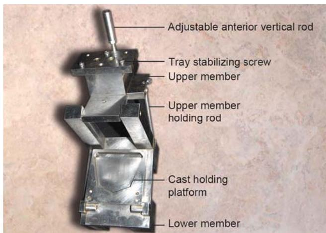
Fig. 2: Inner view of the upper and lower membrane of the impression tray positioning device
