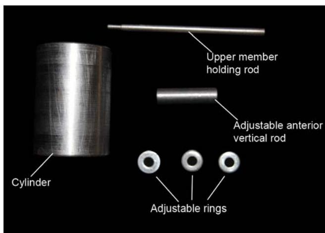
Fig. 3: Detachable parts of the impression tray positioning device
