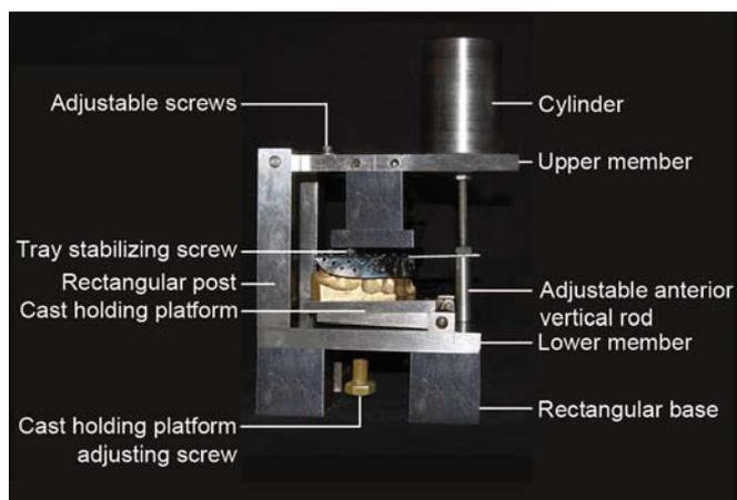
Fig. 1: Profile view of the impression tray positioning device
