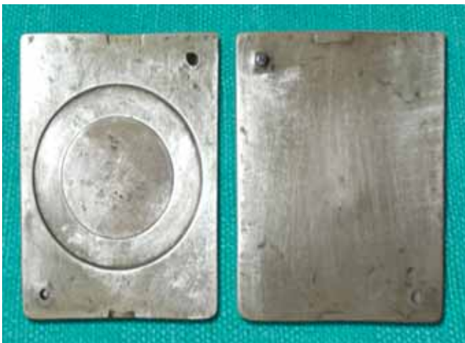
Fig. 5: Brass mold for water sorption samples
