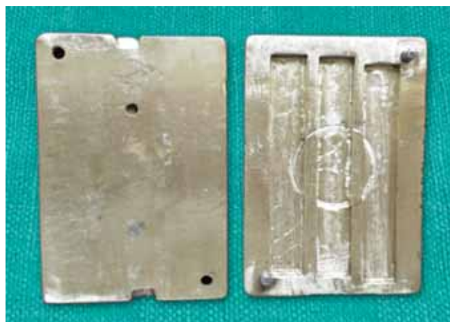
Fig. 1: Brass mold for flexural strength samples
