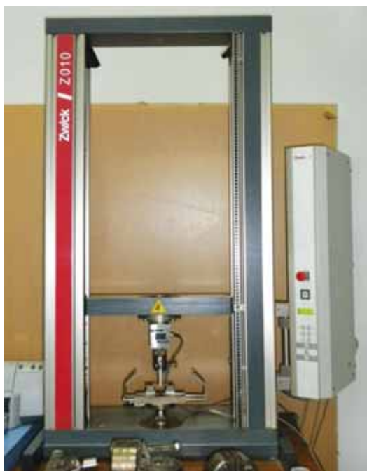
Fig. 2: Sample testing on Zwick-Z010 Universal testing machine
