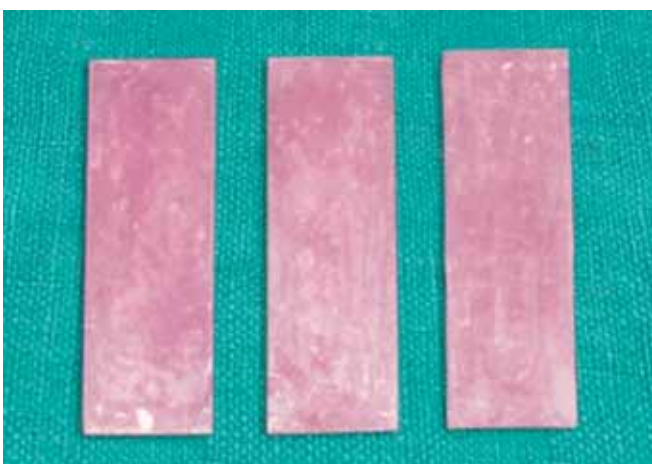
Fig. 2: Heat-polymerized acrylic resin plates
